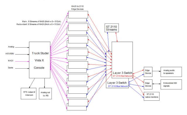
Existing RTS Adam-M Mid-size modular matrix intercom system will be retained for use. This intercom system has SMPTE 2110 interfacing capabilities, however, it is our intention at this time that there will be no tie-in between intercom system and SMPTE 2110 router. This intercom system does not take any embedded audio feeds. IFB feeds are fed by audio console and not integrated into intercom. Audio console Aux sends feed intercom, no mix minus busses are used.
